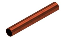
Copper is C12200, Seamless, Light Drawn (H55), Type L, ACR/MED bendable quality tubing, conforming to ASTM B75. The copper tube meets dimensional, chemical, mechanical strength, cleanliness, and eddy current testing requirements of ASTM B280 and ASTM B819 as applicable.
