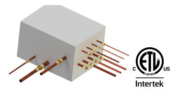
These kits provide the necessary couplings, reducers, and/or caps to connect VRF Branch Selector Boxes to outdoor unit piping and indoor unit piping. Each kit is custom built to match the project system selection lay-out as provided by the customer. The couplings, reducers, flare tube kits, or closed pipe caps are shipped loose for field installation on to the selector box.
