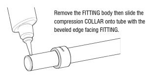
Apply LocTite® to full circumference of tube end. Keep LocTite® 1/8" from end of TUBE and INSERT.
