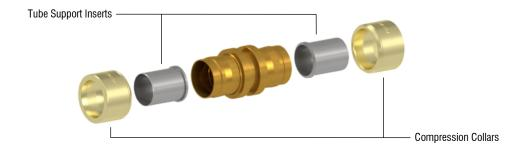
The fittings are permanently connected to the copper tubing by use of a portable, battery operated hydraulic pressing tool, with specially designed, quick-change clamps and clamp inserts. The time required to produces a gas tight connection is significantly less than flame brazing. This cold connection process eliminates the need for high temperature brazing, nitrogen purge, fire watch, and hot work permits. Harmful gases and smoke produced from the brazing process are also eliminated.
