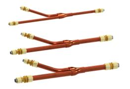
These kits are braze-free alternative to the equipment manufacturer Outdoor Unit Multi Connection Pipe Kits. These outdoor pipe kits provide the necessary Y-Branch fittings, couplings, reducers, to field connect dual and triple frame VRF outdoor units to the refrigerant tubing system by means of permanent mechanical connection. Each kit is custom built to match the project system selection lay-out as provided by the customer.
