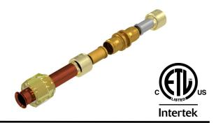
These kits connect copper refrigeration tubing to the mechanical equipment by means of a permanent mechanical seal to a JIS B 8607 Class 2 Flare Stub. To ensure equipment compatibility, this kit is designed to utilize the factory Flare Nut provided with the original equipment.
